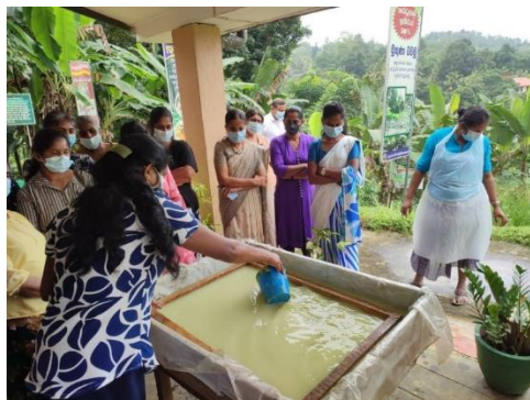
Figure 1. Use of a novel natural rubber latex based binder in manufacture of paper out of the fibers of “Mana” weed
