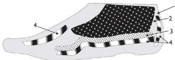
Fig. 6. Schematic diagram of compression moulded prosthetic foot1-Hybrid nanomaterial filled NR nanocomposite, 2- Wooden socket, 3-Canvas belt, 4-4- Nano tructured natural rubber cellular compound
