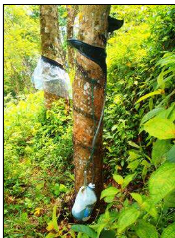
Fig. 2. The device used to measure the stem flow of rubber trees
