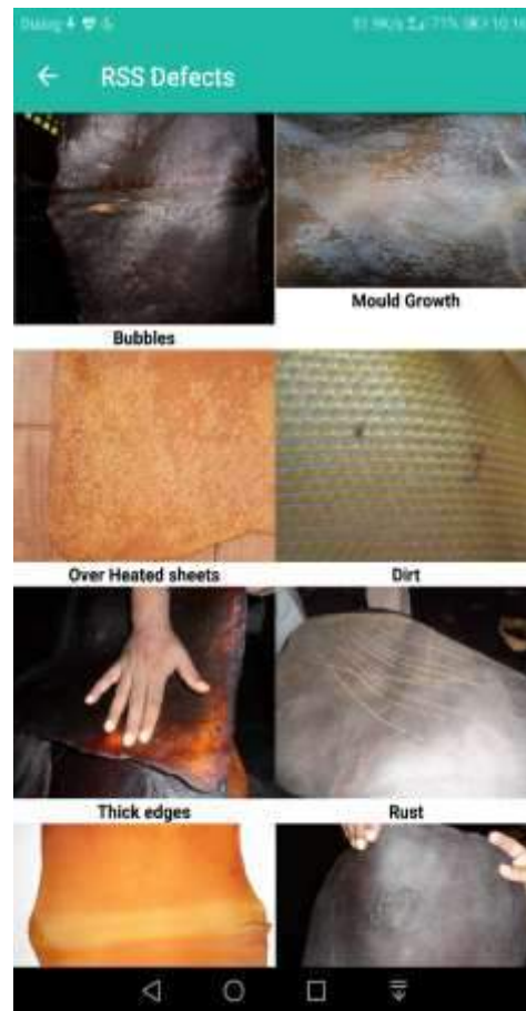
Fig. 16. RSS defect identifier
