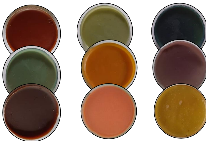
Fig. 10. Natural rubber latex based cast films of different colours produced using five natural materials (D G Edirisinghe, U A Weerasinghe, Ishani Jayaratne and Nushara Nanayakkara)
