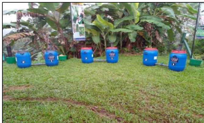
Fig. 3. Pre-treatment system suggested for waste water generated at RSS manufacturing facilities
