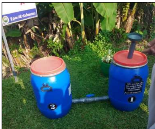
Fig. 22. Mini scale effluent treatment plants distributed among rubber smallholders
