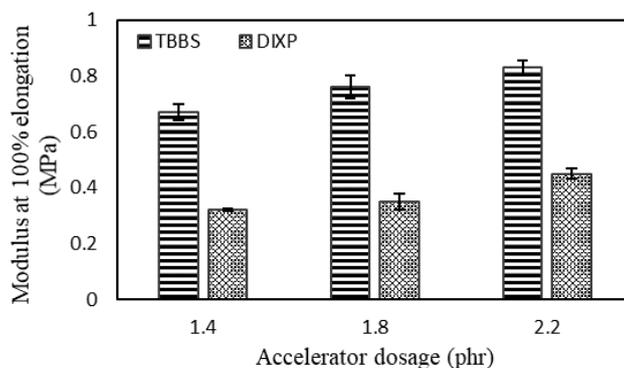
Fig. 12.  $M_{100}$  of the vulcanizates prepared with DIXP and TBBS
