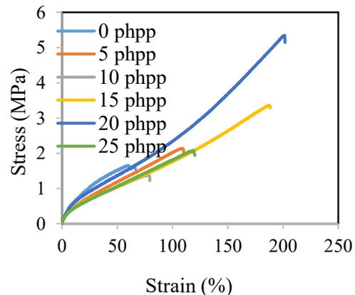
**Fig. 2.** Strain–stress curves of NR/LDPE/wPE composites
