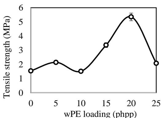
**Fig. 3.** Variation of tensile strength of NR/LDPE/wPE composites with wPE loading
