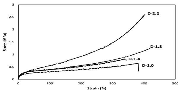
Fig. 9. Stress-strain curves of NR vulcanizates prepared with different TBBS dosages
