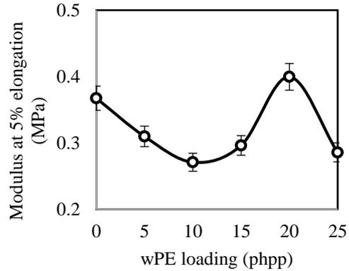
**Fig. 5.** Variation of modulus at 5% elongation of NR/LDPE/wPE composites with wPE loading
