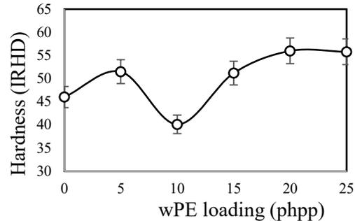
**Fig. 1.** Variation of hardness of NR/LDPE/wPE composites with wPE loading
