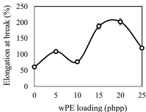
**Fig. 4.** Variation of elongation at break of NR/LDPE/wPE composites with wPE loading
