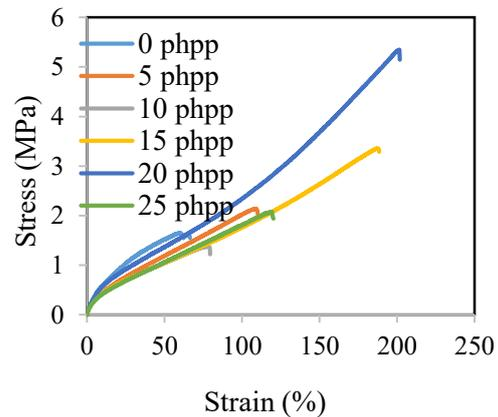
**Fig. 2.** Strain–stress curves of NR/LDPE/wPE composites
