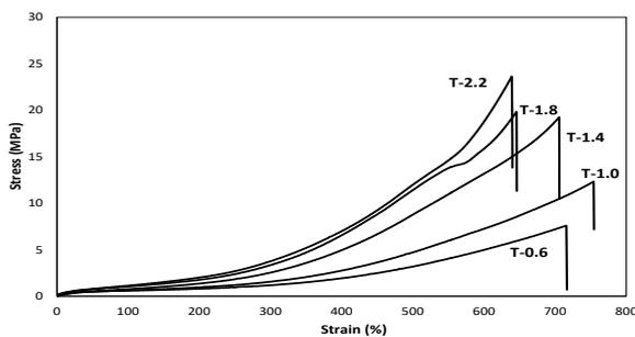
Fig. 8. Stress-strain curves of NR vulcanizates prepared with different DIXP dosages
