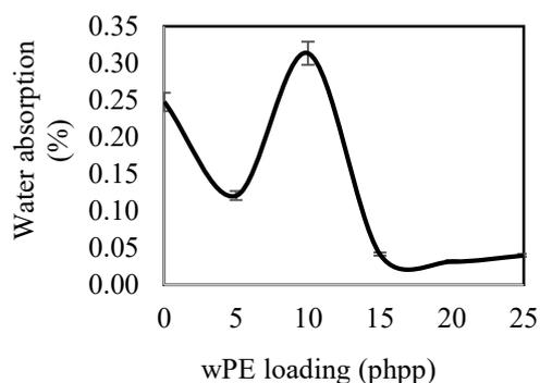
**Fig. 8.** Variation of water absorption of NR/LDPE/wPE composites with wPE loading
