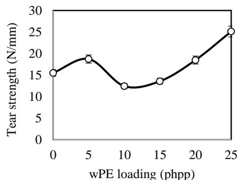
**Fig. 6.** Variation of tear strength of NR/LDPE/wPE composites with wPE loading
