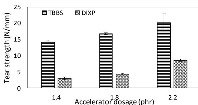
**Fig. 15.** Tear strength of the vulcanizates prepared with DIXP and TBBS
