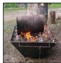
Fig. 7. Biochar preparation in a Barrel
