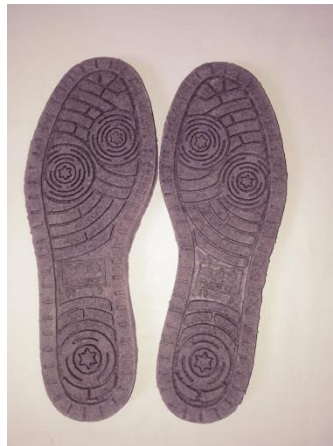
Figure 2: NR based shoe soles produced with durian husk fibres
